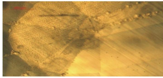
Fig. 4a: Feathers and straight growth lines in untreated natural yellow sapphire
