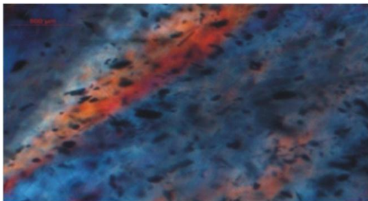
Fig. 6a: Glass filled sapphire showing orange flash effects
